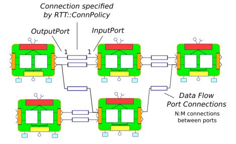
This figure shows that input and output ports can be connected in an N:M way. See Section 4.2, "Setting up the Data Flow" on how to connect ports and which connection policy to choose.
