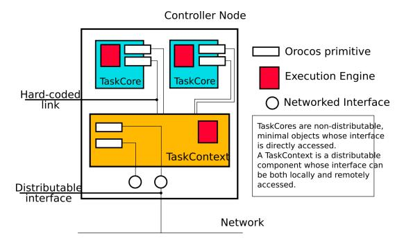
Figure 2.11. Example Component Deployment.
