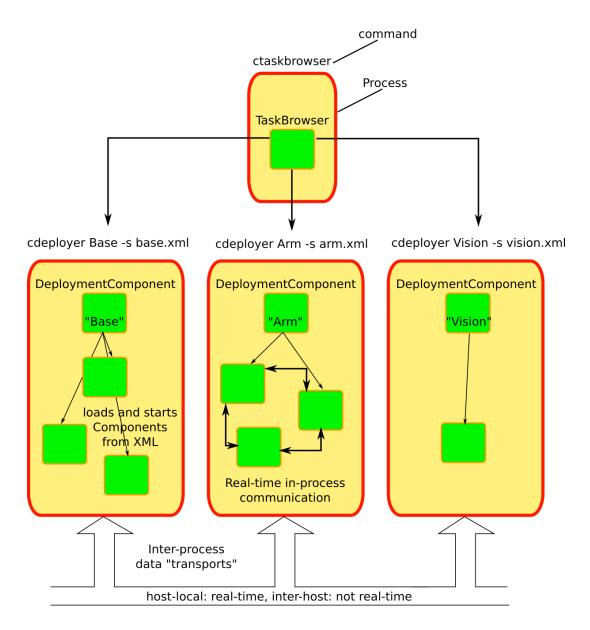
Components are loaded into the process by a deployer, which gets its configuration through an XML file. Communication between processes is transparant to the component, but your data must be known to Orocos (cfr 'typekits' and 'transports'). Most new users start with a single process however, using the 'deployer' application.
