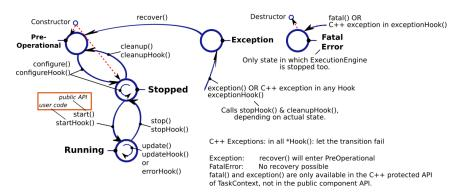
This figure shows the extended state diagram of a TaskContext. This is Figure 2.5, "TaskContext State Diagram" extended with two more states: Exception and FatalError.
