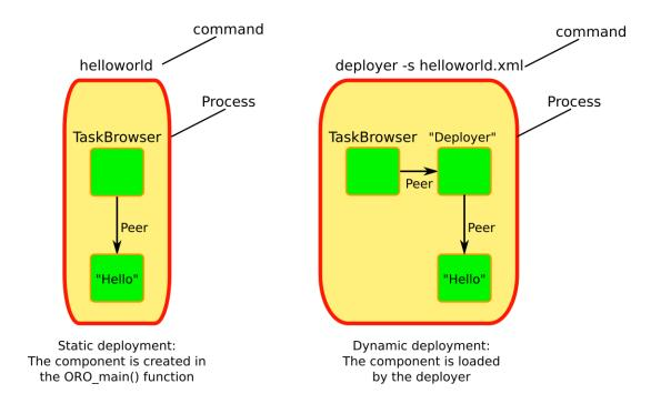
The 'helloworld' executable is a static deployment of one component in a process, which means it is hard-coded in the helloworld.cpp file. In contrast, using the deployer application allows you to load a component library dynamically.
