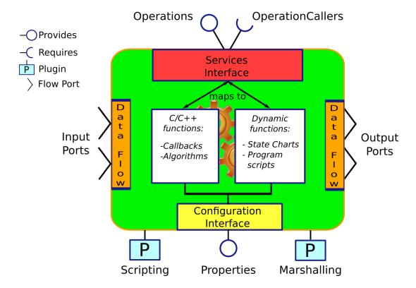
The component offers services through operations, and requests them through operation callers. The Data Flow is the propagation of data from one task to another, where one producer can have multiple consumers and the other way around.
