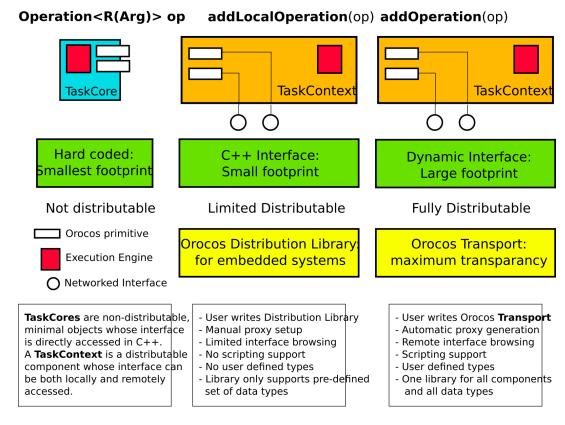
Three levels of using or creating Components can be accomplished in Orocos: Not distributed, embedded distributed and fully distributed.
