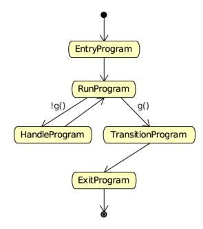
The automatic mode additionally actively evaluates guard conditions. Event reaction remains in effect, but is not shown in this diagram.
